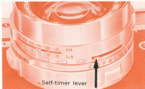
When the self-timer is used, the shutter will be actuated about ten seconds after the shutter button has been pressed. Follow the instructions below :
