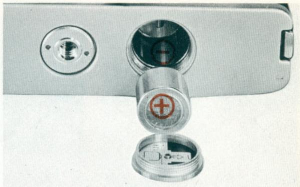
Load the mercury battery in a separate envelope into the battery compartment. Since the mercury battery powers the CdS meter, unless the battery is in position the meter will not function.
