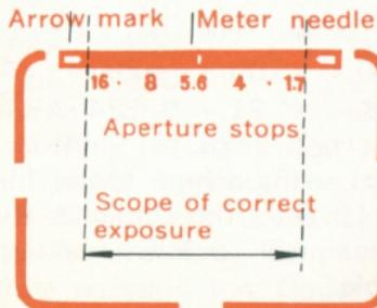
The diagram shown here is the finder for QL 17. In the case of Canonet QL 19, the aperture stop on the right end starts from 1.9.
