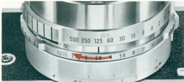
When the AUTO mark of the Canonet S has been removed, the automatic mechanism ceases to function. It is then possible to manually operate the aperture and shutter speed separately. Accordingly, when the effective use of the shutter speed or aperture is desired, or in case it is essential to expose the dark subject for a long time, as well as to regulate the aperture for flash photography, the manual mechanism should be employed. Everything else is operated as usual.
