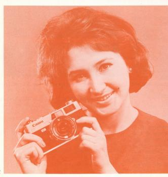
Holding the camera firmly is very important if you want to take a clearly focused picture. Hold the camera in either a vertical or horizontal position, as shown in the photographs. Look through the finder, and adjust the focus while determining the composition. Then, gently press the shutter button.
