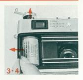
Since no further winding is possible when the end of the film is reached, rewind the film into the original cartridge, as explained below. As the exposed film is naked within the camera, the entire roll will be ruined if the cover is opened before rewinding.
