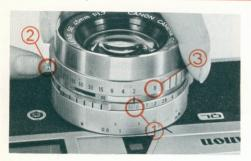
B stands for bulb exposure. Since the shutter remains open as long as the shutter button is being pressed, it is used for long exposures exceeding 1 sec.
