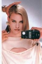
Hold the Flash Meter IV near the subject with the receptor pointing directly at the camera.
