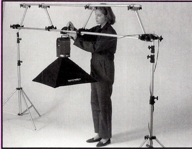
Above: Combitubes used with joint sleeves can make up bridge-like structures of high stiffness. In this photograph a softbox is suspended from the center of a 10-ft. structure. Such an arrangement is inherently stable and far more secure than a boom and counterweight setup.
