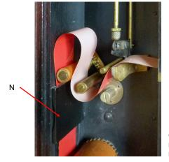
Cutting and nicking mechanism.
