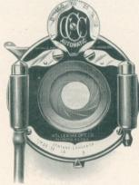
The mechanism is so arranged that after an exposure is completed the shutter automatically sets itself for the next picture. There can never be a question as to "whether the Shutter is set"-it is ready at all times, being released and set simultaneously by either the finger or bulb.
