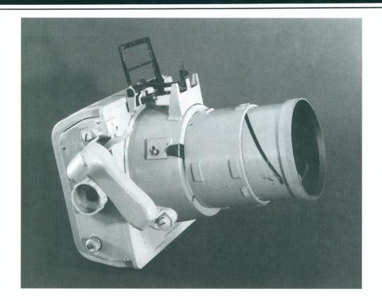
To complement the frontal view on page one, we have both right and left views of our aerial camera. Note the simple sportsframe type finder and sight, perfect for what this unit was meant for. The two large wood side mounted handles make holding the camera secure and comfortable, considering its weight and size. The lens cone collapses and extends with a twisting action
