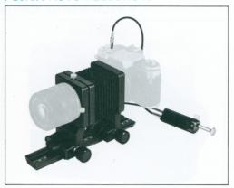
Designed for taking ultra-close-ups, it provides 1-3X magnification in combination with a 50mm normal lens. It is equipped with an automatic diaphragm to allow you to focus with the aperture wide open. Convenience accessories include a focusing rail and a slide copier.
