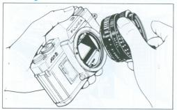
Position the red dot on the lens rear opposite the red dot on the Lens Mount, then push the Lens in and turn it 65° to the right (clockwise). It will lock into position with a click.
