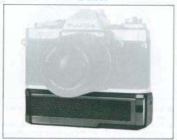
This compact, lightweight unit is attached to the bottom of your camera to wind the film automatically at a rate of two frames per second so that you can concentrate on your subject and won't miss those decisive moments that can easily be lost forever. It will advance the film continuously while the shutter release is depressed or one frame at a time each time the shutter is tripped. It operates on four penlight batteries and a red LED will turn on while the film is advancing.
