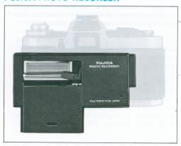
This data back is interchangeable with the Camera Back and is equipped with a hand-writing pen that is interlinked with a "light pen" for printing in data (up to about 30 letters) in the bottom left corner of the picture. The Camera Back can be easily detached by pushing down the hinge pin.
