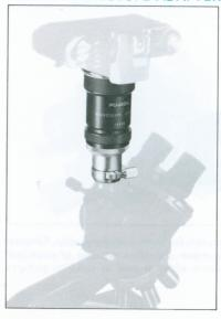
This is used to couple the camera to a microscope to take photomicrographs.
