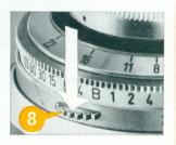
When you have set the light value, for instance 10, you can read off one of the following aperture-speed combinations against the triangle \( \blacktriangle \) index mark (9):
