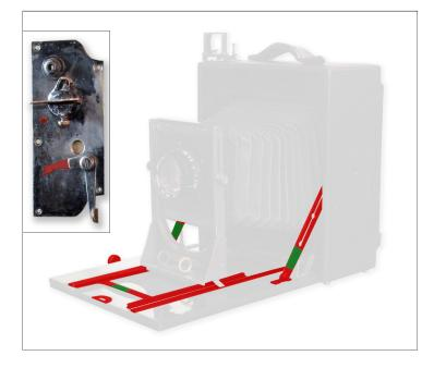
Items in red are from a 4x5 parts camera, and in green, fabricated elements. Closing 4x5 compasses were cut and lengthened by 3 centimeters, made of brass and silver soldered. Insert, parts to be fabricated.
