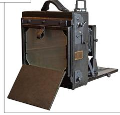
I used the old bellows as a template for a new bellows. I use a synthetic leather from DALBE <a href="www.dalbe.fr">www.dalbe.fr</a>. The handle leather is also from Chapat. I use a 1909 Singer sewing machine for the heavy leather. Another good leather source is <a href="www.cuirdeco.fr">www.cuirdeco.fr</a>.
