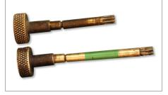
Shown is the modification of the focus knob. At the top is an original 4x5 pre-Anniversary model and at the bottom an original Top Handle 4x5 model. Shown in green are the parts brazed and turned.
