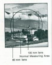
The normal measuring area of the LUNASIX 3 corresponds to a light acceptance angle of  $30^\circ$ . Still narrower angles ( $15^\circ$  or  $7.5^\circ$ ) can be measured when the LUNASIX 3 is used with the Variable Angle "spot meter" Attachment. (See page 27.)
