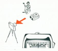
Incident Light Measurement: Move the converter slide (10) so that the spherical diffuser is centered over the round window. The LUNASIX 3 is ready when the converter slide has clicked into position. The LUNASIX 3 is pointed from the subject towards the camera, as indicated by the arrow in the illustration.
