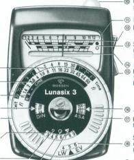
© Converter Slide with spherical diffuser for incident light measurement
