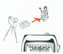
Reflected Light Measurement: Move the converter slide (10) all the way to the right; this uncovers the round window. The LUNA-SIX 3 is ready when the converter slide has clicked into position. Point the LUNASIX 3 toward the subject, as indicated by the arrow in the illustration.
