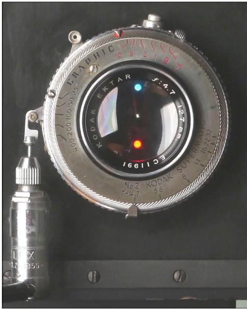
is well, you'll see a blue light at the top, white in the center and red at the bottom. A red light at the top or center means the shutter opened early, a blue light at the center or bottom means the shutter opened late." In operation, the colors don't mean a whole lot. If it's not in sync, you won't get three lights. Top, or top and center, means it's early. Bottom, or bottom and center, means it's late.
