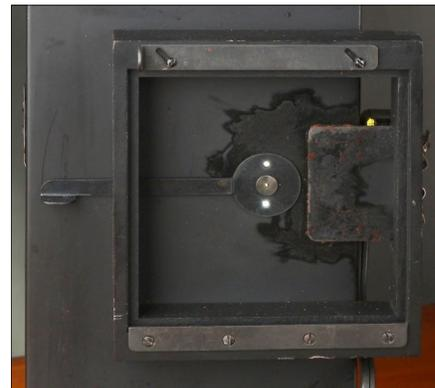
In operation, the lens-board is mounted to the tester. The micro-switch on the right is wired to the trip circuit (behind the red button, on the flash), and the solenoid is wired to the battery case normally. A lever on the tester is set to the center, which opens two small holes behind the lens.
