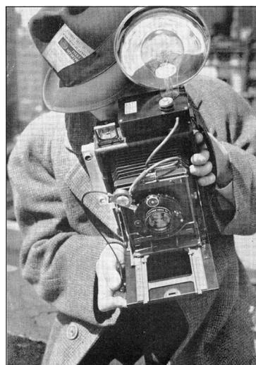
Kalart Micromatic Speed Flash on 4x5 Speed Graphic.
