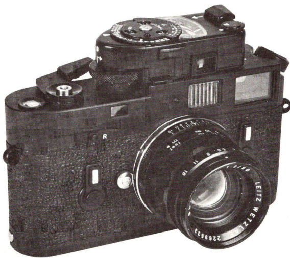
MR-4 meter mounted on a typical M camera such as the M4.
