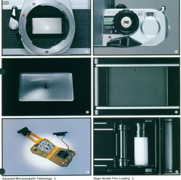
The intricate circuits of this electronic brain hold the key to the MG's high performance and compact dimensions. Using the latest ICs, LSIs and flexible circuit boards, the microcomputer analyses exposure information and sets precisely the right shutter speed with astonishing speed and accuracy.
