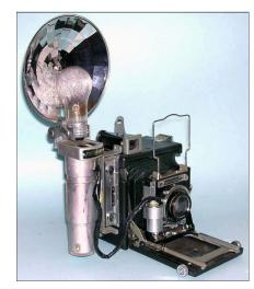
each other and then together as a unit. I put two D batteries in the flash holder, and everything is now working. The coating on the original wires was dry and crumbling. The lens is a Carl Zeiss Jena Tessar 1:3,5 f=10.5cm, and the shutter is a Compur-Rapid. This was the most expensive lens/shutter combination advertised that year at \$142.
