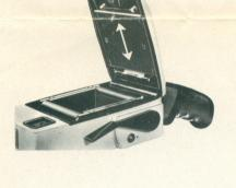
LIFT OUT THE QUICKLOAD FILM INSERT. Place the empty spool on the geared take-up side, the fresh film spool on the feed side (marked "full"); pull the start of the safety paper leader without slack across and thread it into the wide slot of the take-up spool. Advance the leader - by turning the grooved flange on the take-up side - until its starting arrow is lined up with the red arrow on the feed side of the Insert.
