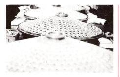
Lenses undergoing Super-Multi-Coating process.
