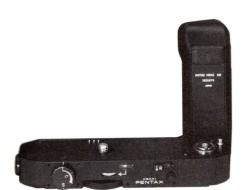
The powerful micro motor of the compact Motor Drive MD, the heart of the K2DMD motor drive system, propels the film at a rate of  $\frac{1}{2}$  -2 fps. Furthermore, a single touch is all that is required to changeover from single-frame to consecutive exposure operation. Also found on this unit are the exposure counter, trigger release, remote control socket, tripod socket, and rewind lever.
