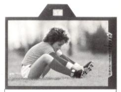
The Viable Viewfinder. In the above example, the following information is available at a glance: The aperture is f/5.6, no compensation is being used, the camera is set to AUTO, the automatic exposure is approximately 1/125, and the subject is properly composed and focused.
