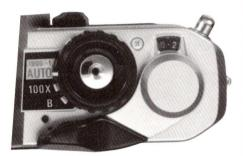
Seiko MFC vertical-run metal focal plane shutter; automatic exposure electronically controlled in stepless range from 1 second to 1/1000 second; mechanical speeds of 1/100 second and B operational without batteries; 3 position shutter mode selector.
