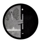
When the meter needle is close to the (+) mark, you will get an over-exposure. If the needle is close to the (-) mark, you will get an under-exposure. In either case, change the shutter speed or the aperture to bring the needle to the center for correct exposure.
