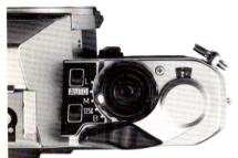
Seiko MFC-E2 vertical-run metal focal plane shutter; automatic exposure electronically controlled in stepless range from 4 seconds to 1/2000 second; full range of 14 manual shutter speed electronically timed from 4 seconds to 1/2000 second, controlled by dual pushbutton action; mechanical speeds of 1/125 second and B operational without batteries; shutter release lock provided; 5 position shutter mode selector.
