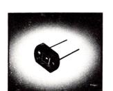
The high performance SPD photosensitive cell (silicon photo diode) installed in the Spotmeter V-FL.
