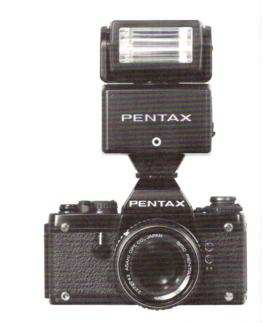
When used in the TTL mode with the Pentax LX, the film plane measured automatic exposure range of the new AF-280T Automatic Electronic Flash is from 0.8 feet to 65.6 feet with an f/1.4 lens and ASA 100 film.
