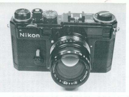
ABOVE IS THE BLACK SP WITH THE S3 BELOW. NOTE THE TWO TYPES OF SELFTIMER LEVERS, THE CHROME RE-WIND AND WIND LEVERS AND THE SHUTTER SPEED DIALS. ALSO THE STRAP LUGS ARE CHROME.
