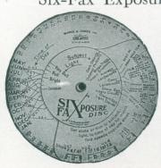
This is the most accurate and simplest exposure calculator made, is based upon the six essentials which determine correct exposure.
