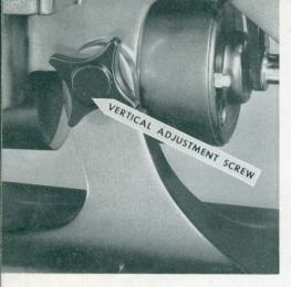
SCREW on the base and tilting the Kodascope, then tightening SCREW.
