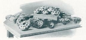
Lens discs in their shells ready for grinding
