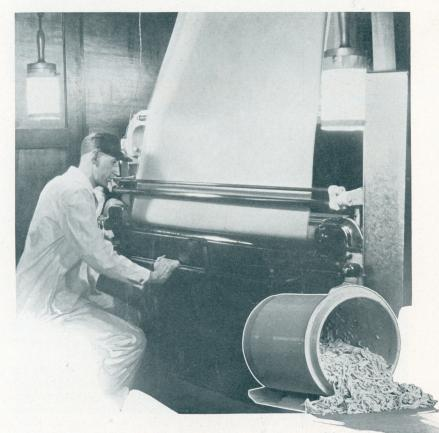
Coating the light sensitive emulsion on the film base. Insert shows the shredded emulsion before it is melted for the coating machines
