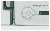
Calculate "F-numbers" by dividing the guide number shown in the table by the distance from the camera to subject. Set F-number in F-number scale by turning Auto/Flash selection dial.
