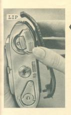
Close the back: Insert the LIP at the narrow end of the camera back cover into the channel on the camera body near the take-up spool. Press down the other end of the cover until it clicks into locked position.
