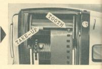
Slowly rotate the TAKE-UP spool until the narrow end of the film is nearly wound on, and the perforation of the full width "leader" part of the film is engaged on the SPROCKET. The film must run between the edge GUIDES.
