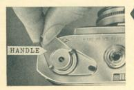
Crank the HANDLE clockwise until a resistance is felt; the film is now rewound into its magazine. Fold the HANDLE back into closed position and press it down until the rewind LOCK clicks into place.
