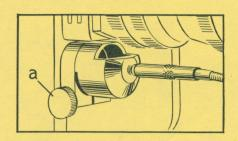
On Bolex H-16 Rex cameras equipped with Rexofader, single frame exposures can be made by attaching a Bolex Universal cable release in the threaded hole of the blade #10 of the Rexofader (see Rexofader instructions). This arrangement works satisfactorily only on cameras equipped with a grooved and knurled release button (above serial #172201). The buttons are easily interchangeable and owners of cameras below this serial number should exchange the old button for the new type.
