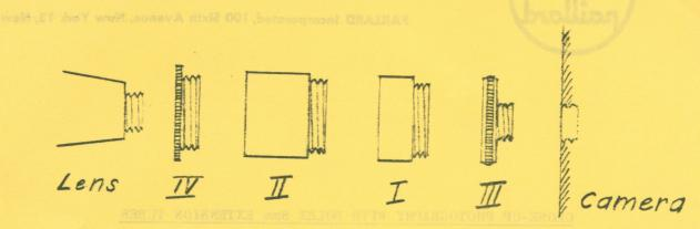
They are used only with telephoto lenses but a variety of magnifications can be obtained since the rings can be combined in four different ways:
