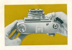
possible and repeat this procedure with the rapid transport lever and release lever until the number 36, 20 or 12 is opposite the fixed mark, according to the length of the film.
