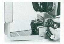
■ Align the base end of the lens mount board to the orange-white line on the magnification scale of the bellows and secure it in position with the lens clamping knob.
