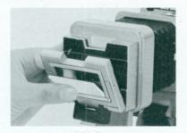
Removal of the Diffusion Glass This diffusion glass will be removed from the film holder when the illuminator incorporates its own light diffusion device.
