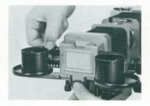
by moving the film holder up or down. Normal positioning is obtained by aligning the red dots on the film holder and arm. To adjust the horizontal position of a film strip, push the button lock and pull the film to the right or left. The opening of the film holder can be adjusted by the adjusting knob. A clockwise turn makes the opening wider, and a counterclockwise turn makes it narrower.
