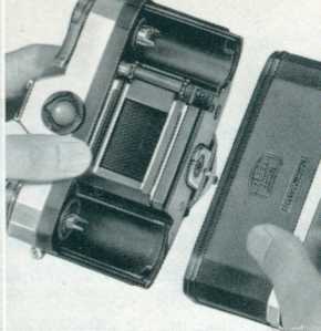
Figs. 2, 3 With your left thumb push the back of the camera downwards (fig. 2) and lift it off with the right hand (fig. 3.)
