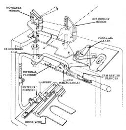
14. The Super has a high-precision builtin rangefinder. The rangefinder cam operates the focusing scale indicator on the stop of the camera, so that the scale always the lens matches used. Shown below is the Pacemaker rangefinder, which is the same system used in the Super Graphic, with a few changes.
