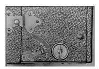
Figure 8. Start-stop and speed selector levers on governor type camerae
