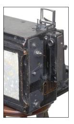
Even more gray painted hardware, and they even replaced/refinished the bed struts! Note the Anniversary style infinity stops and focus scale (coded X14 and designed for a lens of 159.7mm). The bright aluminum focus scale is homemade.
