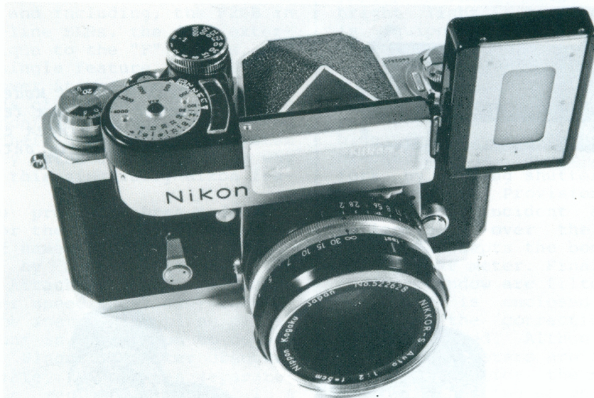
An early Nikon "F" fitted with a boosted Model I and the first version of the Nikkor-S 5cm f2.0 lens. This is what a metered "F" outfit purchased in 1959 would look like. If the booster attachment looks familiar to RF fans, its because it is the identical item! When the booster is attached to the Model I, the horizontal incident plate cannot be removed without first detaching the booster. This inconvenience was later eliminated by designing the plate to slide on vertically on the 3.
