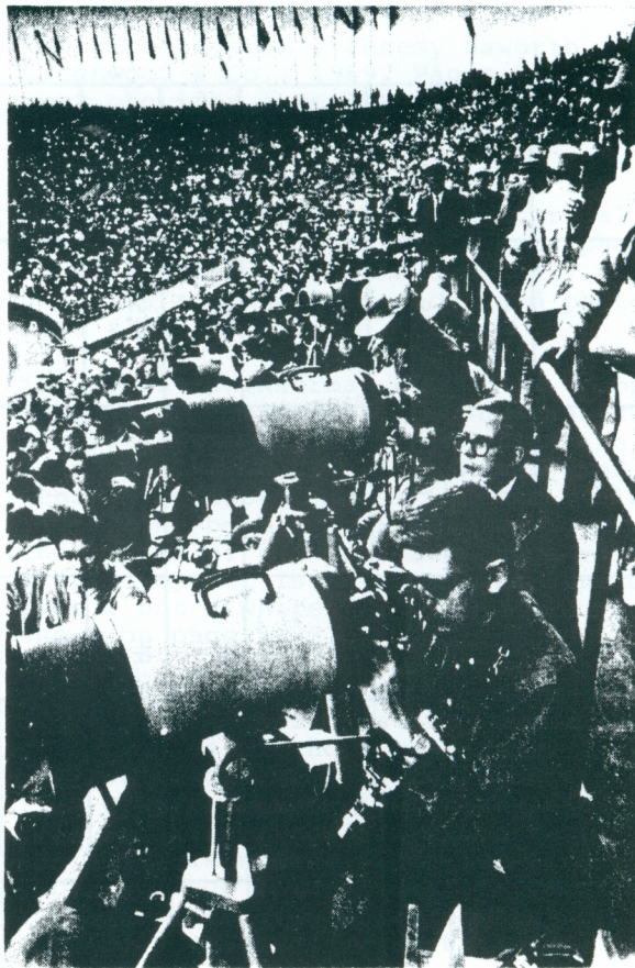
"Big Bertha" catadioptric lenses used with Nikon cameras for sports photography at 1964 Olympic games in Japan.
