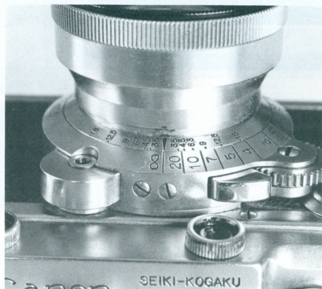
A close-up view of the special Nikon designed bayonet focusing mount used on the Hansa and Seiki Canons. A similar inner bayonet mount would be used much later on Nikon's own camera!
