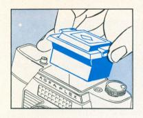
Open and close the waistlevel hood viewfinder by the knob on the lid. If the image is not visible in the viewfinder operate the rapid transport lever.
