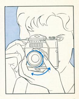
ing ring. You may also hold the camera with the right hand, supporting it on the palm of the left hand, and turn the focusing ring with thumb and index finger of the left hand, as shown in the illustration on page 23.
