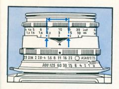
If you select an aperture and shutter speed combination in which f/11 is opposite the black dot and then set the focusing ring to 10 metres (= 30 feet), with the Color Solinar lens you will then obtain a depth of field from about 16 feet to infinity. If the camera is focused on 3 metres (= 10 feet) the sharp zone will be from about 7 to 17 feet.
