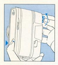
Press in locking button, pull out rewinding knob to the first stop and turn in direction of arrow.
