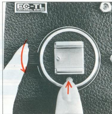
a. To reduce camera vibration to the absolute minimum during shutter release action, especially when the picture image is greatly enlarged, it is possible to lock the mirrors out of the way before releasing the shutter. This will ensure that the picture is free of camera shake and that fine details will be captured clearly, in the picture.
