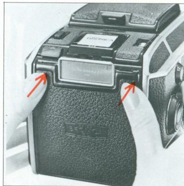
h. Close the back cover of the film back, by pressing the top end of the cover strongly against the film back. A slight click will be heard as the back cover automatically locks.
