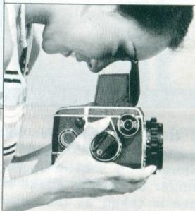
⑦ Once the preselected shutter speed setting is illuminated, release the shutter while checking composition and focus on the focusing screen.
