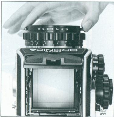
The aperture ring of the standard lens has numbers from 2.8 to 22 on it, which are the f/numbers and indicate the size of the lens opening, when these numbers are opposite the aperture index.
