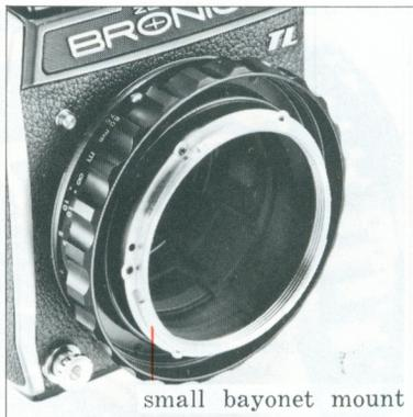
a. Interchangeable lenses which can be used with the small bayonet mount on the focusing ring, are the 40 mm, 50 mm, 75 mm, 80 mm, 100 mm, 150 mm and 200 mm focal length lenses.
