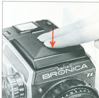
b. To attach the finder on the camera body, simply place the finder lightly into place in its frame on top of the body. Then push down and towards the rear, at the same time, and the finder will catch.
