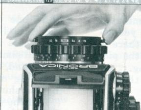
⑥ If it is not the pre-selected shutter speed setting, then adjust the aperture ring in the required direction to obtain the required shutter speed setting.
