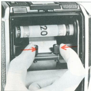
f. Hold the two center knobs pressed inwards and insert the film holder insert into the film back.
