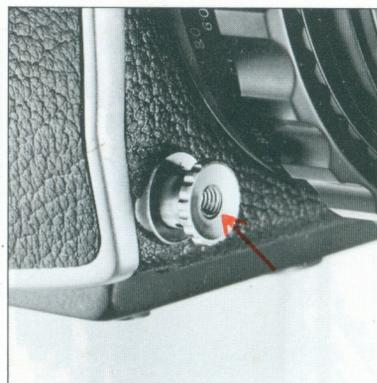
c. The cable release can also be screwed into the socket of the shutter release button and used to release the shutter. The use of the cable release will help minimize camera vibration and give you pictures with greater sharpness and details.
