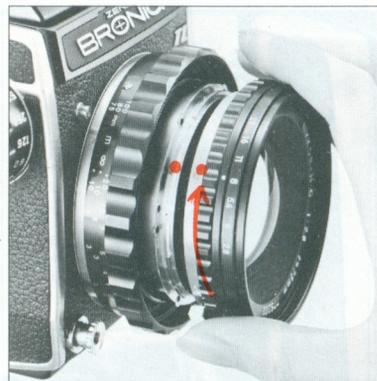
b. To attach the above interchangeable lenses to the small bayonet mount, first, rotate the focusing ring fully clockwise so that the red dot on the outer rim of the small bayonet mount is exposed.
