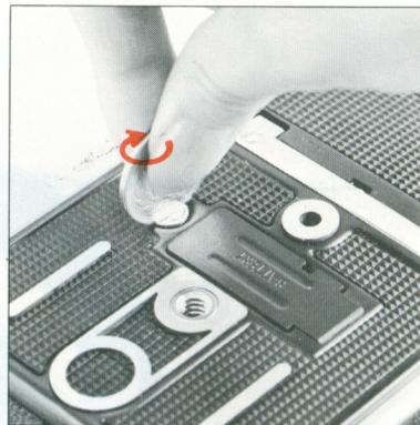
b. To load the battery, open the battery chamber with a coin, or similar object. Insert the coin into the slotted battery chamber button and turn slightly in the arrow-indicated or clockwise direction. The cover of the battery chamber should spring open.
