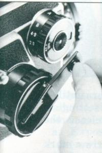
③ Turn the film winding knob/crank two full turns, which will advance the film, cock the shutter and switch in the metering system.
