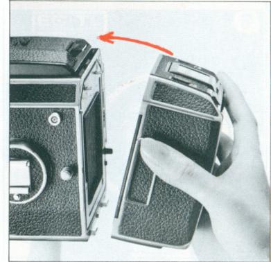
b. To attach the film back to the camera, simply place the bottom edge of the film back against the protruding open hinges on the camera back. Then, press the film back firmly against the camera body until a loud click indicates that the film back has been securely connected. Finally, pull out the dark slide, which will complete the attachment.
