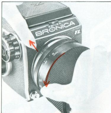
f. Lenses or focusing units attached to the camera body are detached in the same manner as the focusing ring.
