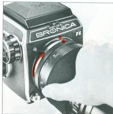
e. Lenses with the large bayonet mount, as well as the common rear focusing unit for the longer telephoto lens heads, are attached in the same manner as the focusing ring. Insert the lens or focusing unit so that the red dots on the lens and bayonet mount are lined up. When well-seated, rotate the lens in the clockwise direction until it stops and the focusing ring release button pops up, indicating that the lens or focusing unit is securely engaged.
