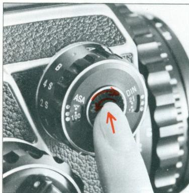
b. To set the film speed, simply press the ball of your finger or thumb against the central dial and rotate the film speed scale until the required ASA film speed (or DIN film speed) is aligned to one of three color-coded film speed indexes around the shutter speed selector ring.
