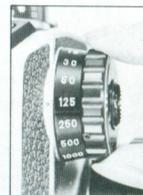
a. If the main subject is not in the center of the finder area and the contrast between the background and the main subject is very great, on AUTO, point the camera (lens) at the main subject for the exposure measurement. Then, transfer the indicated shutter speed setting to the shutter speed scale and take the picture by setting the exposure manually, which will give much better results.
