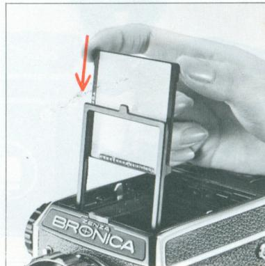
b. To insert the new screen, simply slide it in all the way, with the side marked "TOP" on the top surface side. When inserted fully, simply push the frame down into position, which should lock it into place. However, the frame will not lock into place if the screen is not inserted fully.
