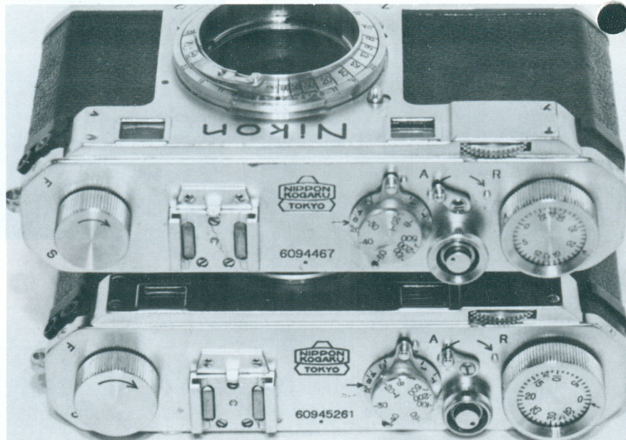
Top-If the original number for 60945261 was actually 6094526, then 6094467 would seem to be very close and should be quite similar if not identical. Yet it is very different!! Besides the shutter guards, they have different castings & 6094467 also has the later type knobs. Bottom-All three cameras lined up for comparison. No two are identical, which is one reason why the early Nikon S can be so interesting.
