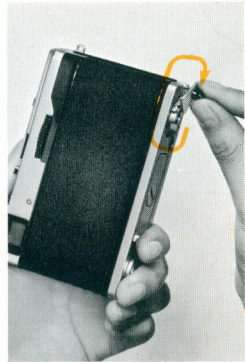
7 After film is completely exposed, rewind the film into magazine and remove. (See page 18.)
