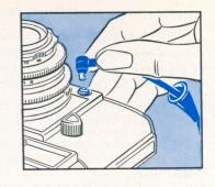
In many cases, particularly with indoor photography, a flashgun will be needed to supplement the available light and for this your Super Solina is provided with a flash contact. You merely slide the flashgun (such as the Agfa KM or Agfalux flashgun) on to the accessory shoe of the camera and attach the flash lead to the contact (see illustration).
