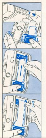
Open camera back by pulling the catch in direction shown by arrow.
