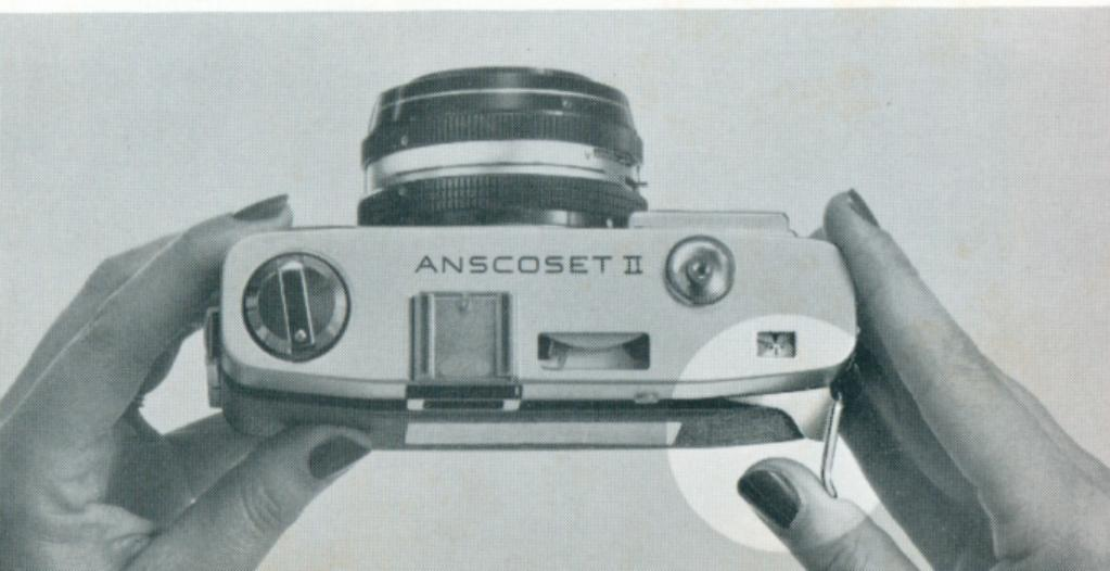
The film rewind knob (No. 1) should turn counterclockwise as the film is advanced; if it does not, it indicates that the film was not properly attached to the take-up spool. Open the camera again and reconnect the film, making sure that the film is taut and that the sprocket teeth are engaged in the film perforations.
