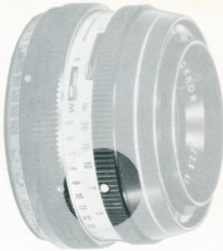
**3** Focus the lens and note the camera-to-subject distance on the footage scale (No. 15) as shown by the position of the white index dot (No. 17) on the lens focusing ring.
