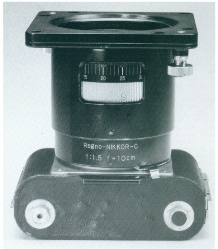
Bottom right-Fig3..Top view of X-Ray outfit, showing detail of fine-tuning adjusting ring on lens barrel. Note thickness of the metal jacket which encases the lens.
