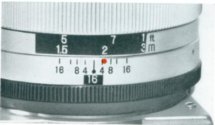
Infrared photo index mark is used for focusing the camera when infrared film and red filter are used. After the subject distance has been determined, the camera to subject distance must be further aligned with the red dot.
