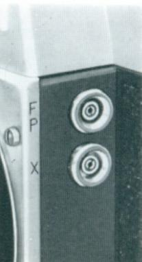
Two separate terminals are provided for flash synchronization FP and X. The upper terminal should be used for FP type flash bulb operation. The synchronization is fully automatic for all shutter speeds, no adjustment is required. For use with "FP" Flash Bulb.
