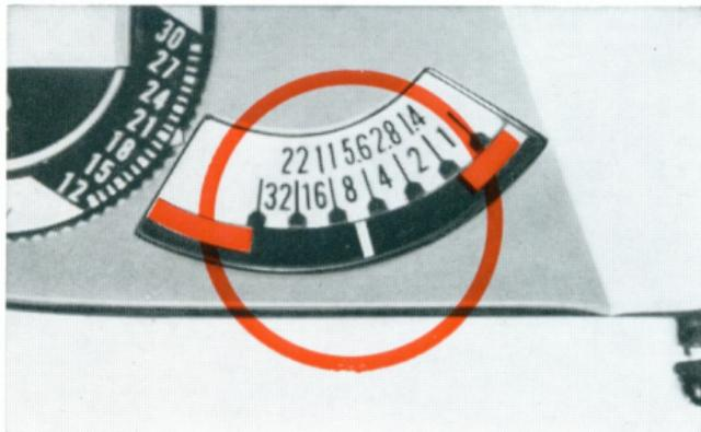
Aim the camera at the subject, the red indicator needle in the Exposure Meter will then show the proper f/stop number.
