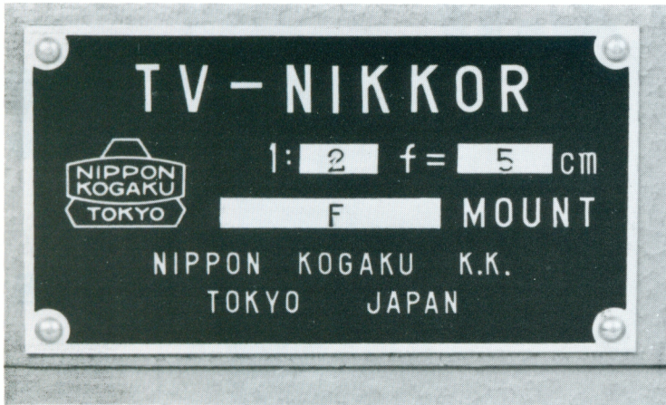
Fig. 2..left..Closeup shot of identification tag. Note the absence of a serial number for this particular lens, and the misleading "F" mount reference!
