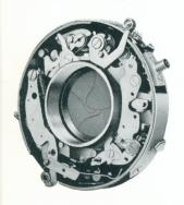
The five blade action of the shutter of PETRI 1.9 gives you accurate readings from 1 to 1/500 second, and includes a bulb setting. The shutter also has a built-in self-timer and is equipped with M.X.S. synchronization which is adaptable to all kinds of flash bulbs and electoronic flash.
