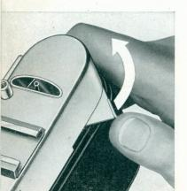
One full movement of the lever tensions the shutter, and advances the film and the film counter. A spring then returns the lever to its original position.
