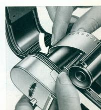
Before closing, the loaded camera must appear as shown in the illustration on the right. The film lies flat in the film track, with the teeth of the transport sprocket engaging the film perforations
