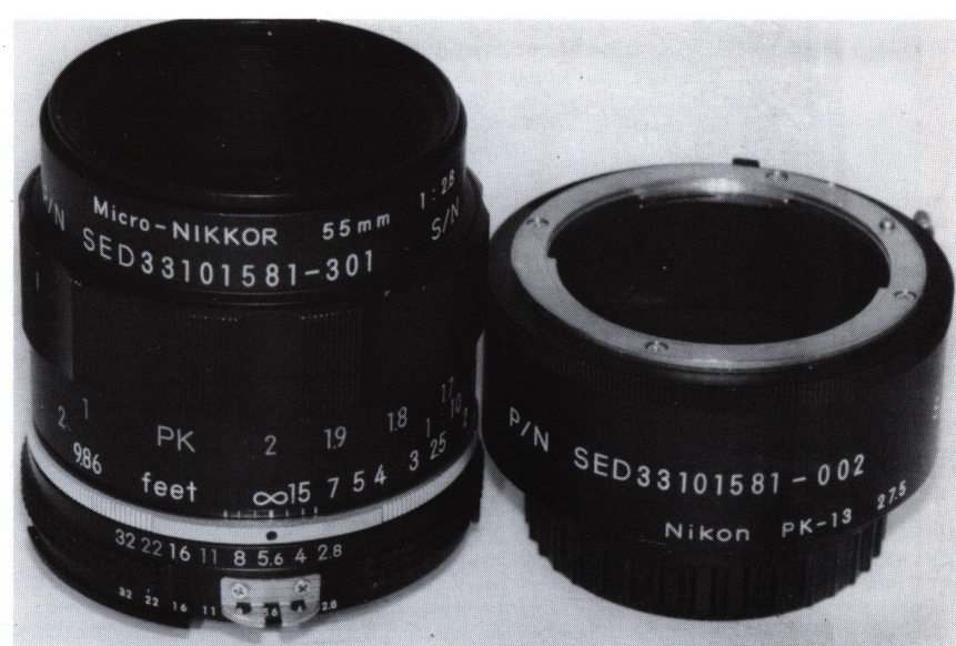
Fig.23-Unlike the other lenses only the focusing ring is matte-black while the rest of the barrel is identical to the standard lens. Near the front rim are engraved the identification numbers.. P/N SED33101581-301 and S/N 10. However, in this case there are two extra digits after the S/N which are not painted in. It actually reads S/N 10 09! (Again the -301 suffix is present as well as the #10!) A proper PK-13 ring is present in this set and it is finished in a matte-black, but not quite as dull as the other two lenses. Its identification numbers are P/N SED33101581-002 (the main number is identical to that on the lens) and S/N M10! It is possible that the "M" harkens back to the previous rings for the Micros that were known as "M" rings. However, like the lens, two extra unpainted digits follow the S/N, which actually reads as S/N M10 01. All engravings on this ring are in white.
