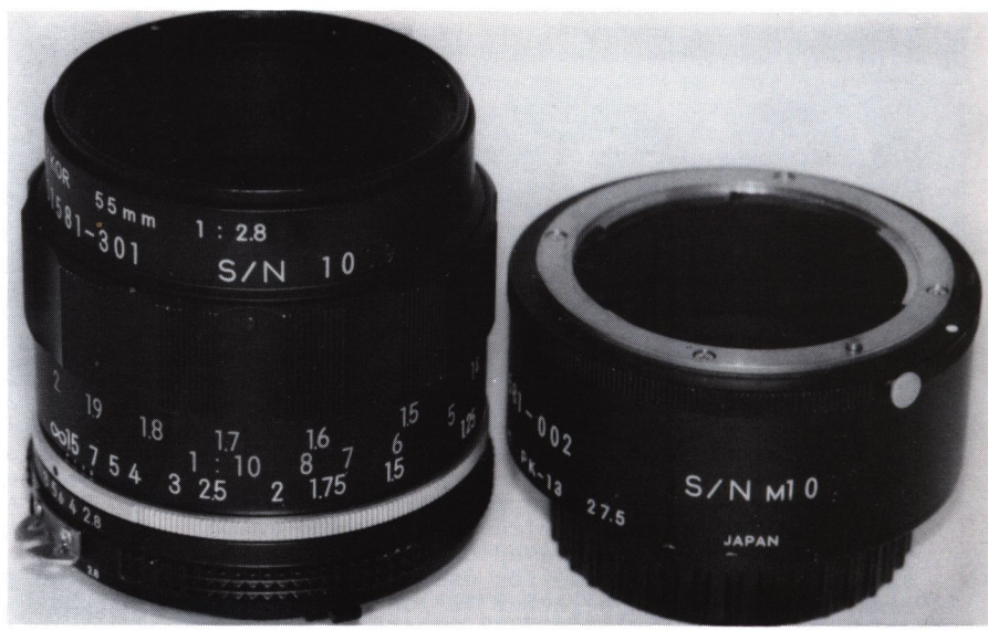
Fig.23-Unlike the other lenses only the focusing ring is matte-black while the rest of the barrel is identical to the standard lens. Near the front rim are engraved the identification numbers.. P/N SED33101581-301 and S/N 10. However, in this case there are two extra digits after the S/N which are not painted in. It actually reads S/N 10 09! (Again the -301 suffix is present as well as the #10!) A proper PK-13 ring is present in this set and it is finished in a matte-black, but not quite as dull as the other two lenses. Its identification numbers are P/N SED33101581-002 (the main number is identical to that on the lens) and S/N M10! It is possible that the "M" harkens back to the previous rings for the Micros that were known as "M" rings. However, like the lens, two extra unpainted digits follow the S/N, which actually reads as S/N M10 01. All engravings on this ring are in white.
