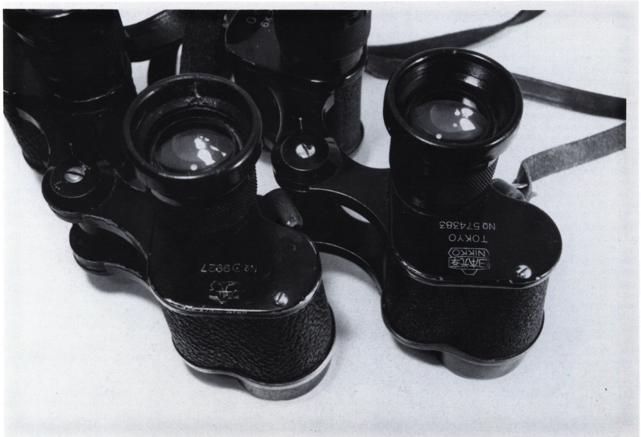
Fig#4-Bottom...On the right are N-K made "Orion" 6x24 glasses from the Occupation era. Compare this to its military counterpart (left) made a few years earlier for the Japanese Army. Both are identical with the exception that the military "Nikko" shows a reticle in its field of view.
