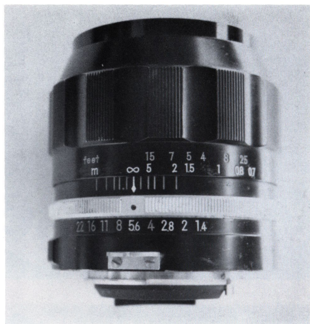
The upper 2 photos are of the DUMMY 35mm/f1.4 Nikkor #350287. The diaphragm ring is frozen at f5.6 and no leaves are present. Only the front and rear elements are evident. Note that "DUMMY" is engraved on the rear surface near the bayonet lugs. R. Keyishian
