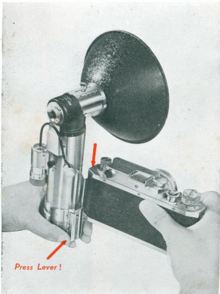
**2nd Step** — When properly housed terminals will coincide and Lock clicks over camera bracket.
