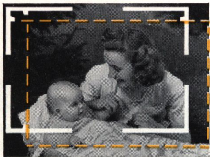
CLOSE-UPS: Dotted lines show what will appear in final picture relative to what is seen in finder.
