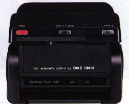
For TTL Auto mode, the flash head back panel reverses.
