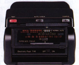
For normal Auto, there is a choice of F4, F5.6 or F8 lens apertures. For Manual, there is a selection of GN45, 32, 22, 16, 11 and 8 guide numbers (ISO/ASA 100, meters).
