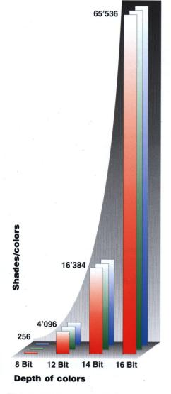
The greater the color depth of a system, the more accurately can individual tones be rendered. The greater the respective color depth, the smaller the effects of rounding-off errors during the various steps of image manipulation.
